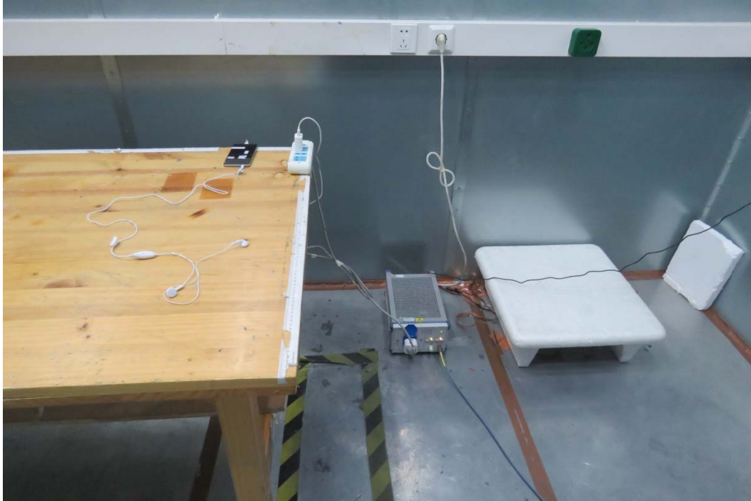
Picture 3 Conducted Emission Test Setup
