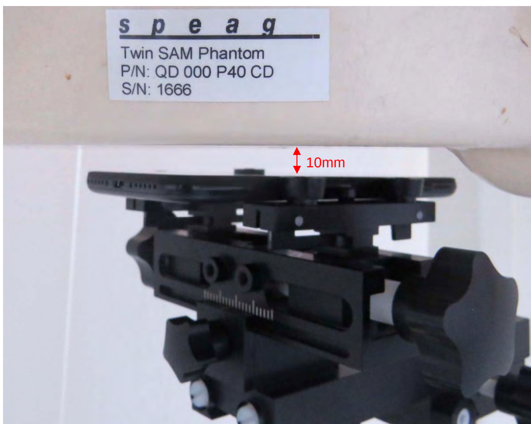
Picture 21: Front Side, the distance from handset to the bottom of the Phantom is 10mm
