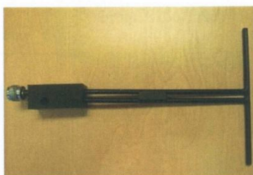
Figure 1 – MVG COMOSAR Validation Dipole
