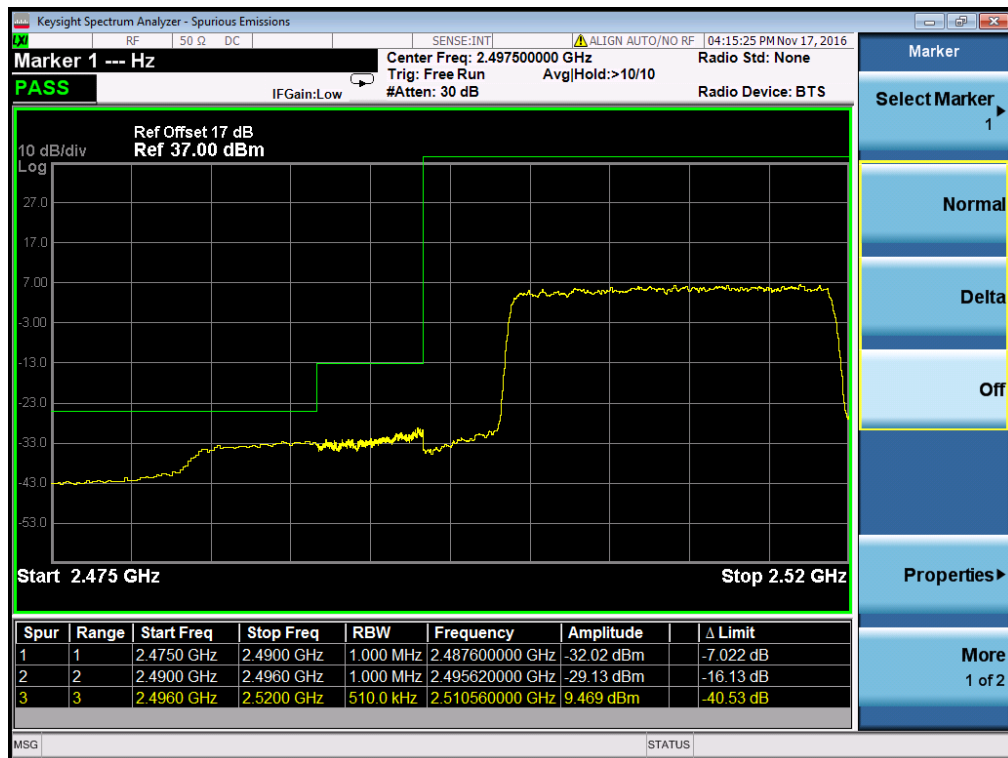
Lower Band Edge Plot for QPSK -RB Size 100, RB Offset 0
