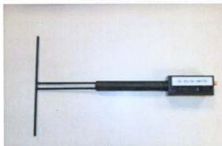
Figure 1 – Satimo COMOSAR Validation Dipole
