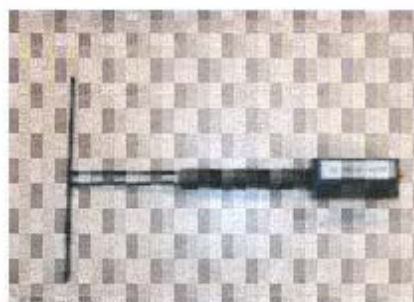
Figure 1 – Satimo COMOSAR Validation Dipole
