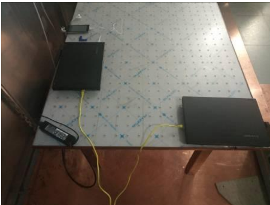
Conducted Emissions Test Setup (with laptop)
