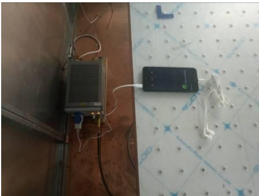
Conducted Emissions Test Setup (with charger)
