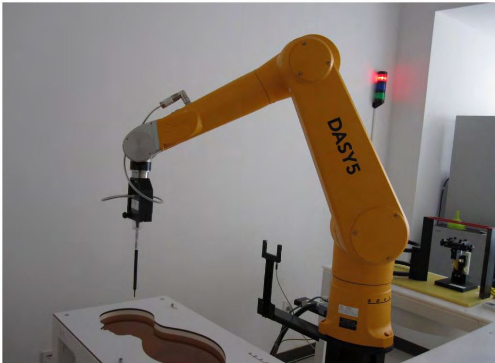
Picture C.1: Specific Absorption Rate Test Layout
