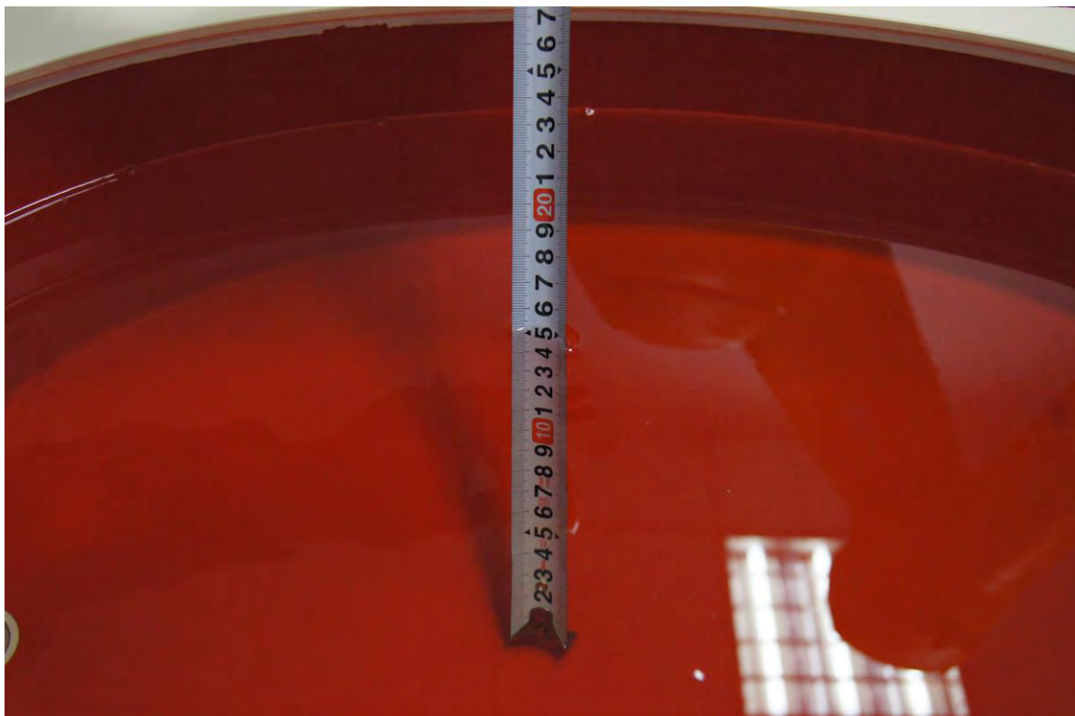
Picture C.2: Liquid depth in the flat Phantom (835MHz) (15.1cm deep)
