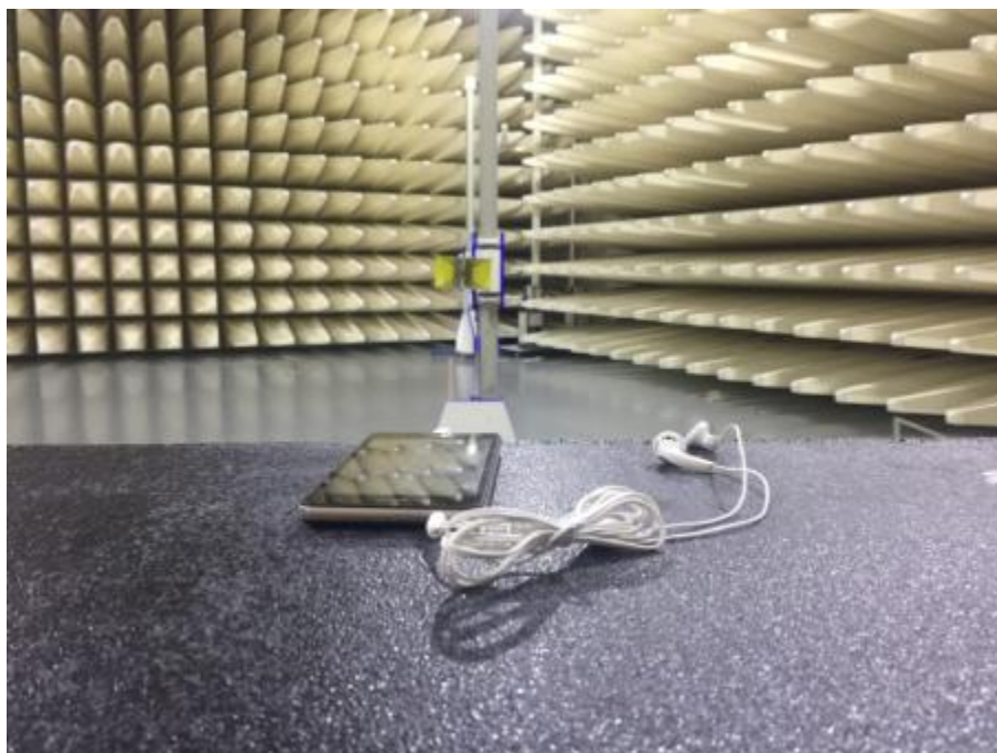
Spurious Radiated Emissions Test setup (1GHz~25GHz)
