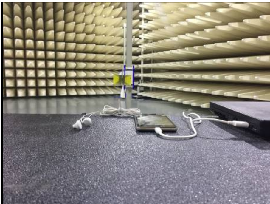
Pic6.Radiated Emissions Test Setup (with laptop)
