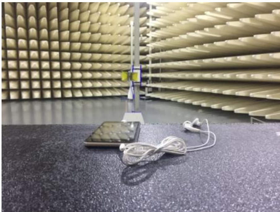
Pic5.Spurious Radiated Emissions Test setup (1GHz~25GHz)
