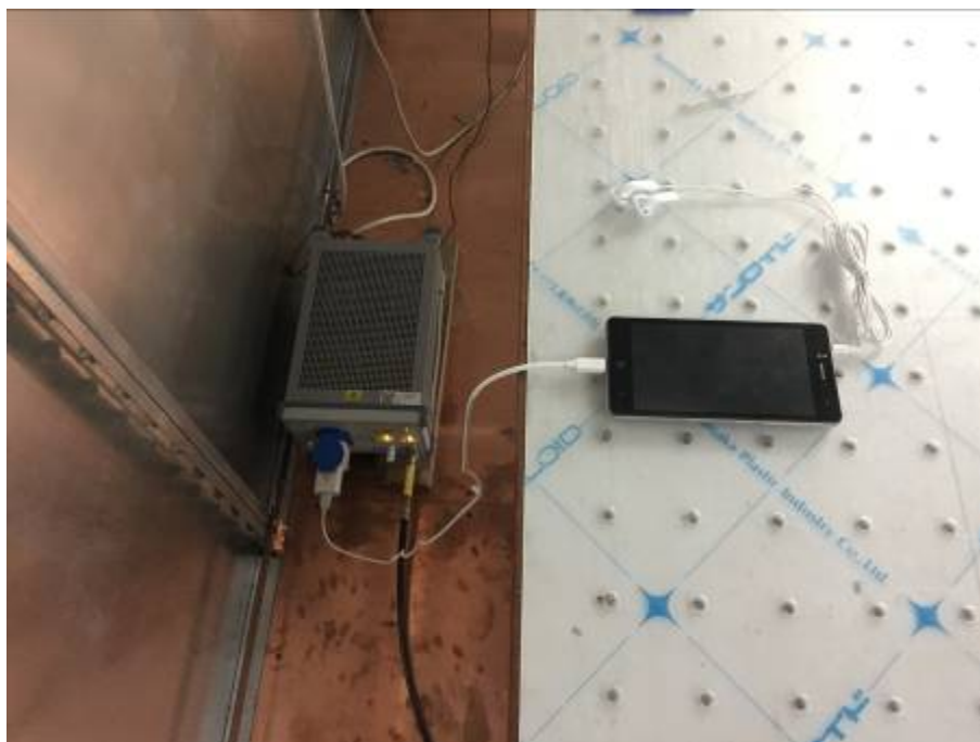
Pic9. Conducted Emissions Test Setup (with charger)
