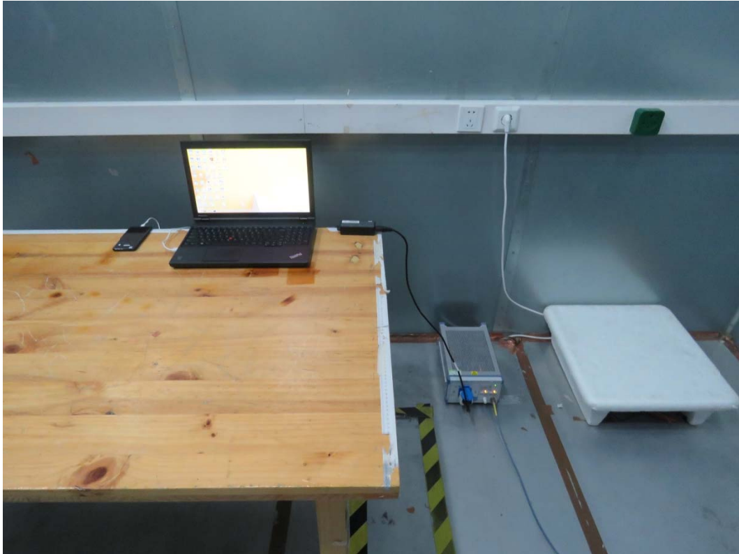
Picture 3 Conducted Emission Test Setup
