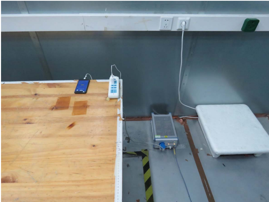
Picture 3 Conducted Emission Test Setup
