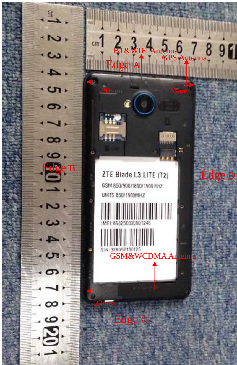
Fig. 3 Position of the antennas
