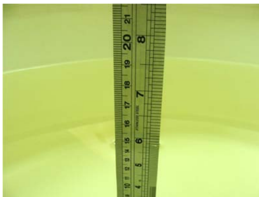
Fig 6.1 Photo of Liquid Height for Body SAR
