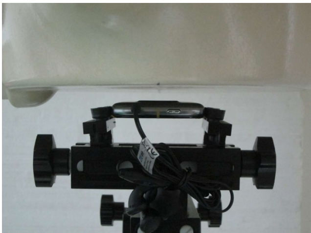
Back with headset, Test Separation 1 cm
