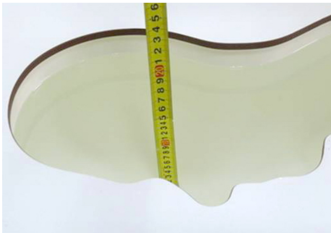
Picture 14: Liquid depth in the head Phantom (2600 MHz, 15.4cm depth)
