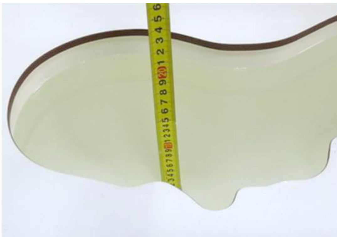
Picture 10: liquid depth in the head Phantom (1900 MHz, 15.3cm depth)
