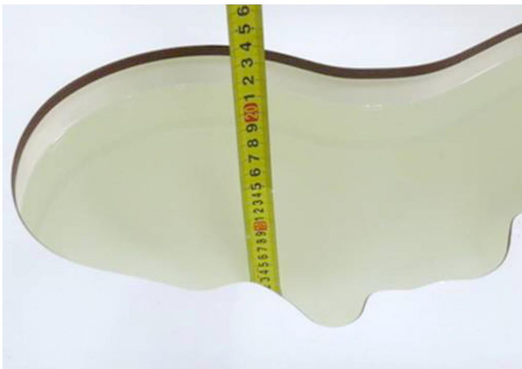
Picture 8: liquid depth in the head Phantom (1750 MHz, 15.3cm depth)
