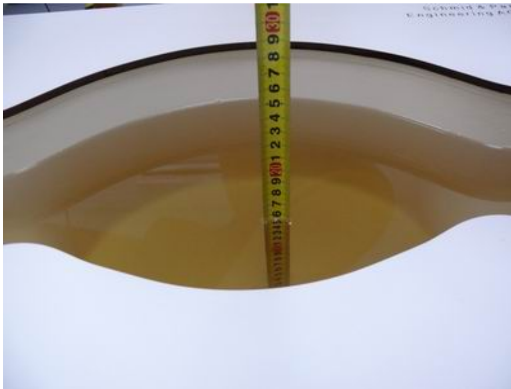
Picture 5: Liquid depth in the flat Phantom (835MHz, 15.4cm depth)
