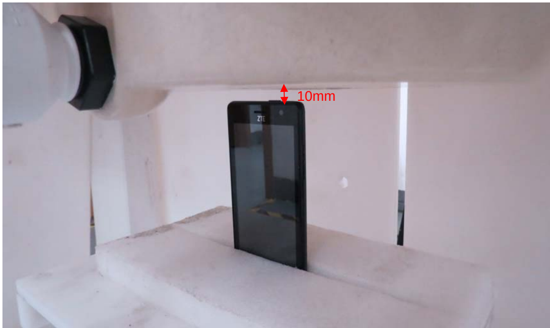
Top Side, the distance from handset to the bottom of the Phantom is 10mm
