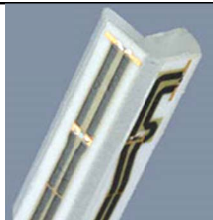
Fig 5.2 Photo of E-field Probe
