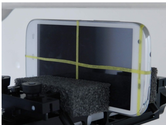
Left side, Test Separation 1 cm
