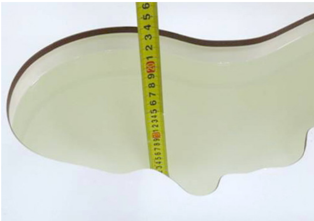
Picture 12: Liquid depth in the head Phantom (2450 MHz, 15.4cm depth)
