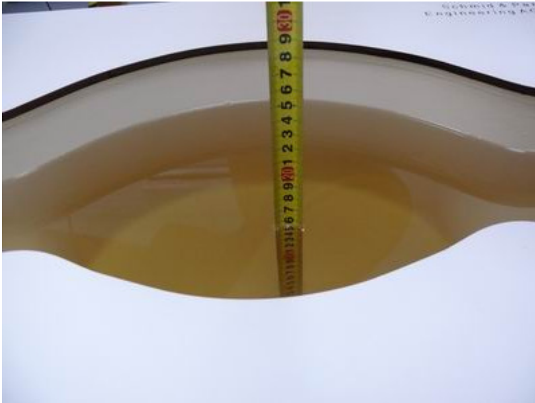
Picture 5: Liquid depth in the flat Phantom (835MHz, 15.4cm depth)
