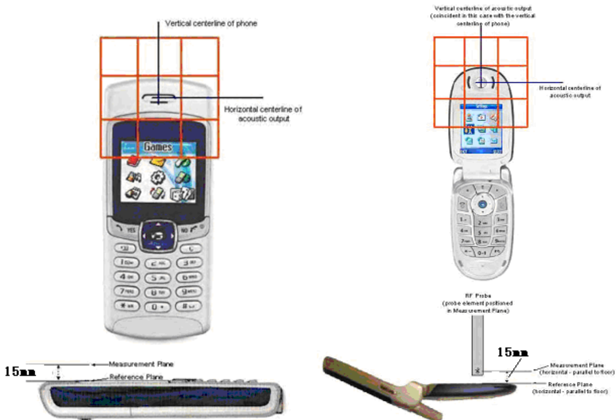
Figure 4 WD reference and plane for RF emission measurements
