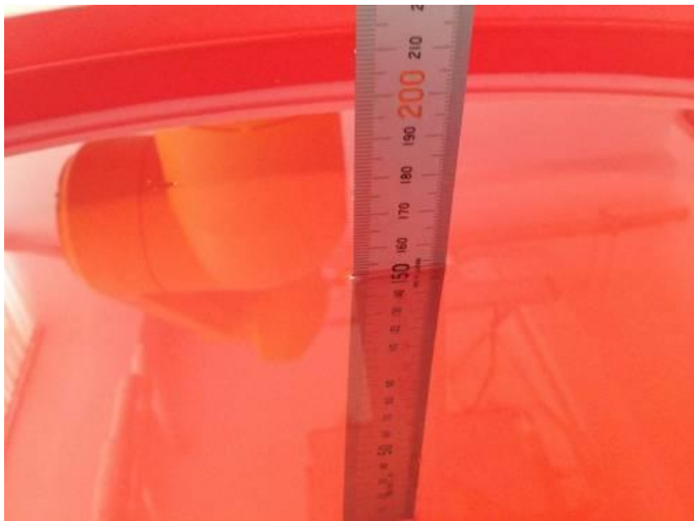
Picture 7-6 Liquid depth in the Flat Phantom (2450MHz) (depth=15.2cm)
