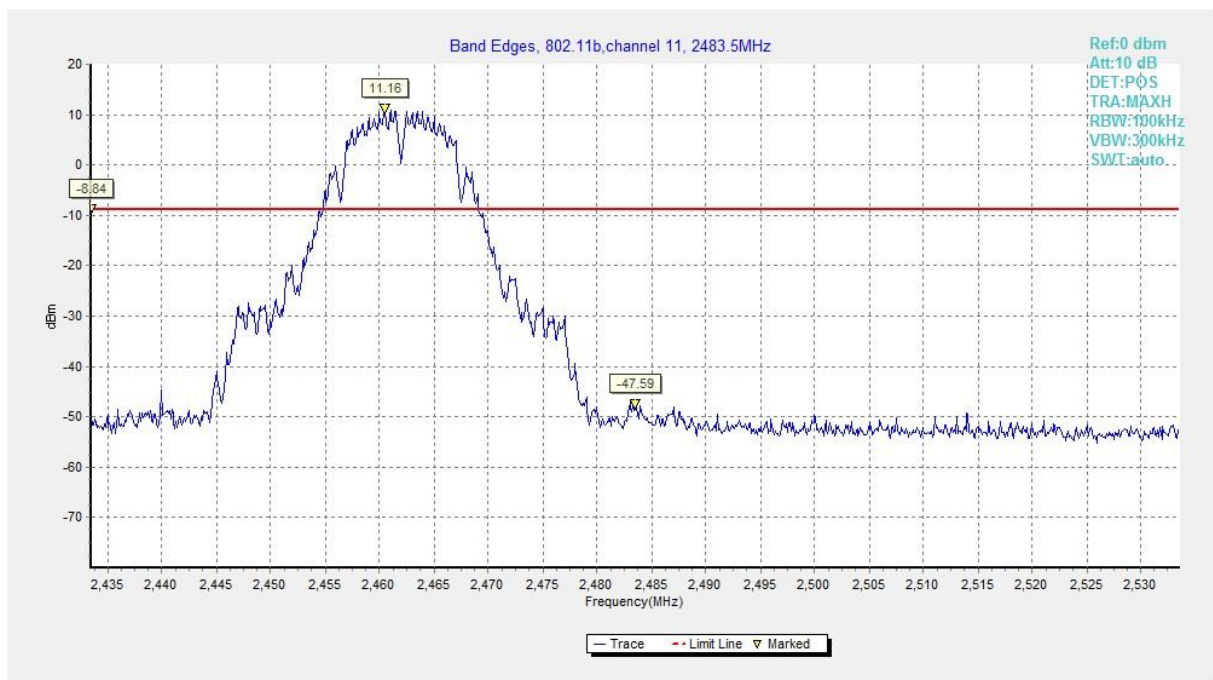
Fig.A.5.2 Band Edges (802.11b, Ch 11)
