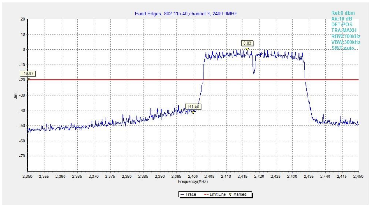
Fig.A.5.7 Band Edges (802.11n-HT40, Ch 3)
