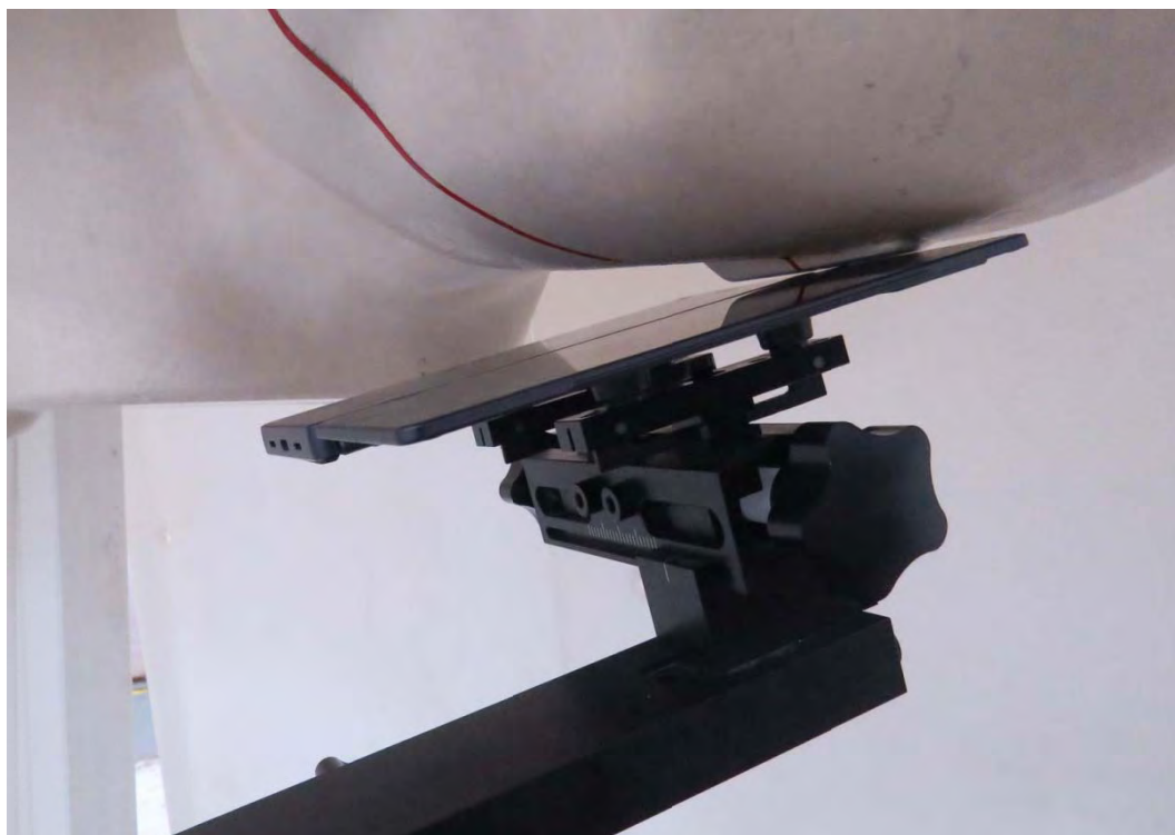
Picture 17: Left Hand Tilt 15 Degree Position For Double Screen Mode
