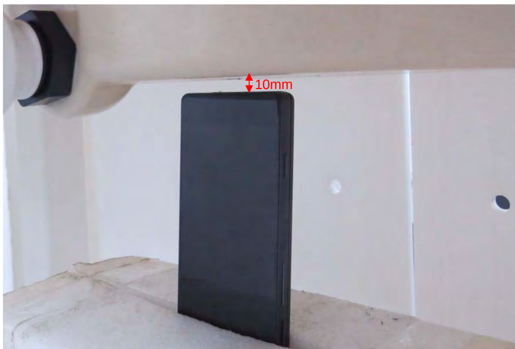
Picture 25: Bottom Side, the distance from handset to the bottom of the Phantom is 10mm For Single Screen Mode
