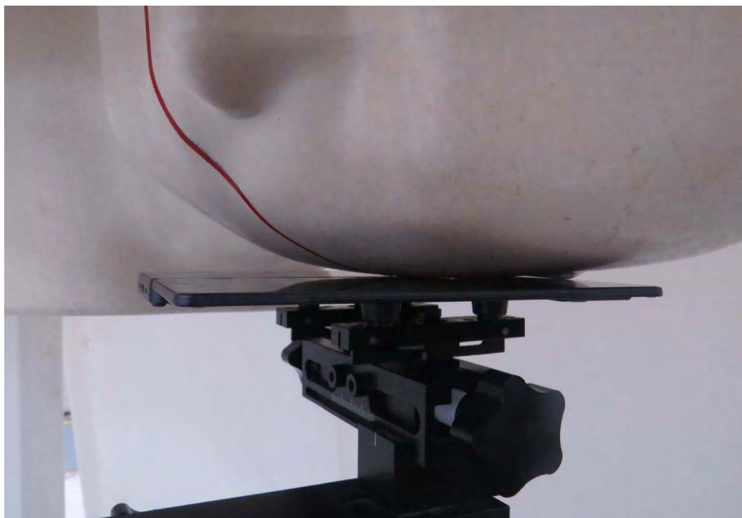
Picture 16: Left Hand Touch Cheek Position For Double Screen Mode
