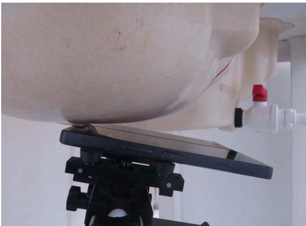
Picture 19: Right Hand Tilt 15 Degree Position For Double Screen Mode
