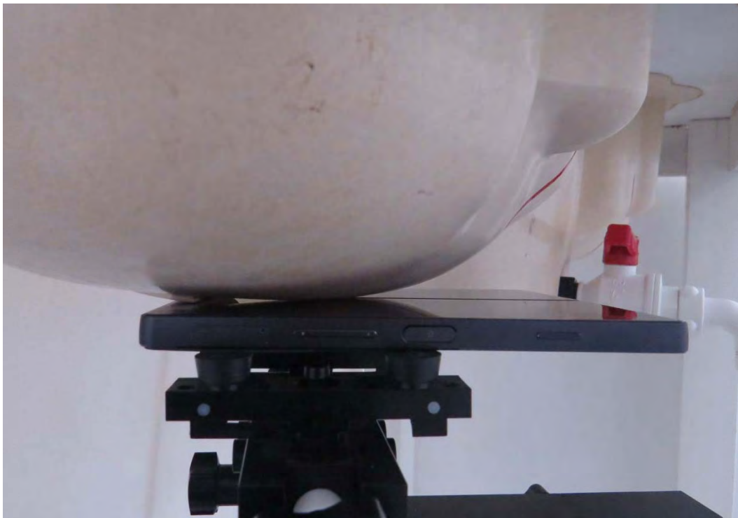
Picture 18: Right Hand Touch Cheek Position For Double Screen Mode
