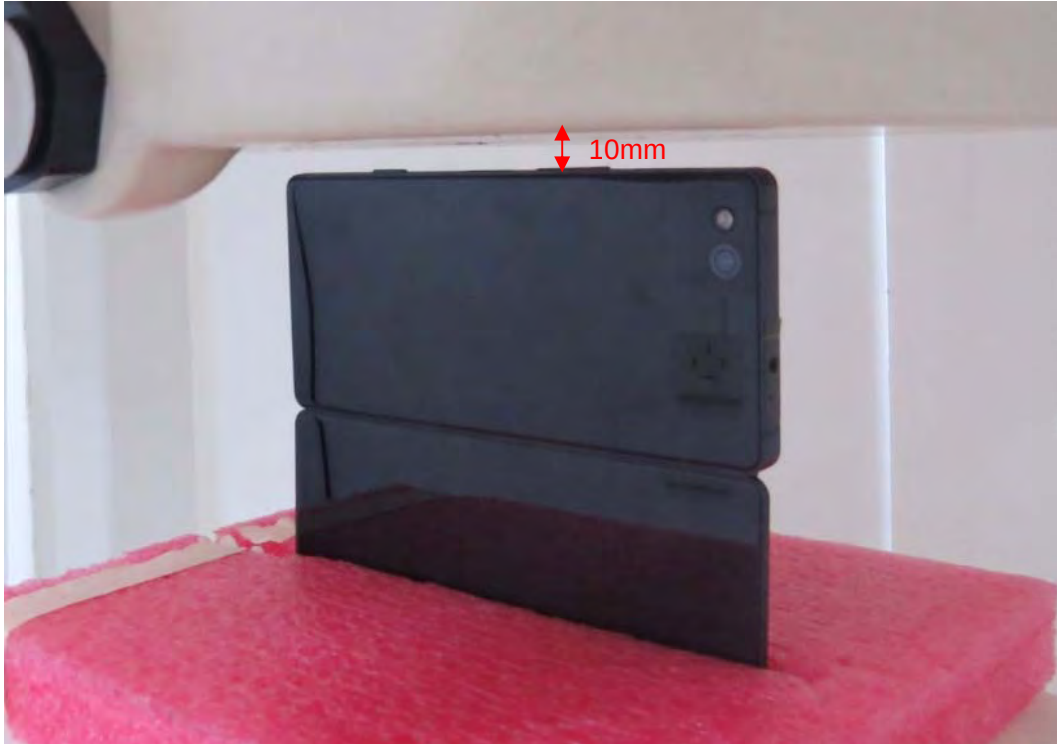
Picture 24: Left Side, the distance from handset to the bottom of the Phantom is 10mm For Double Screen Mode
