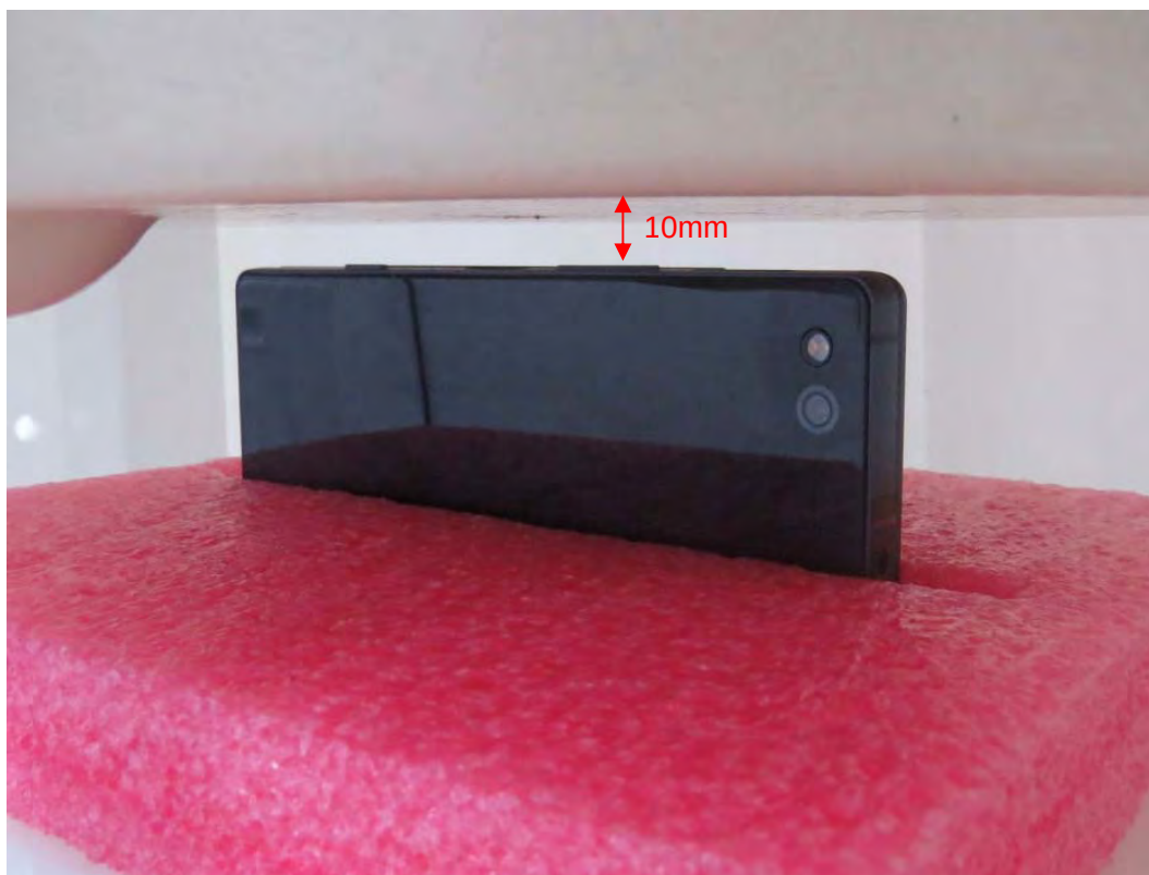
Picture 18: Left Side, the distance from handset to the bottom of the Phantom is 10mm For Single Screen Mode
