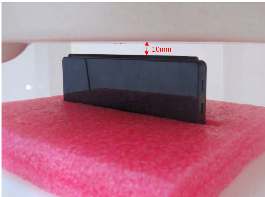
Picture 19: Right Side, the distance from handset to the bottom of the Phantom is 10mm For Single Screen Mode
