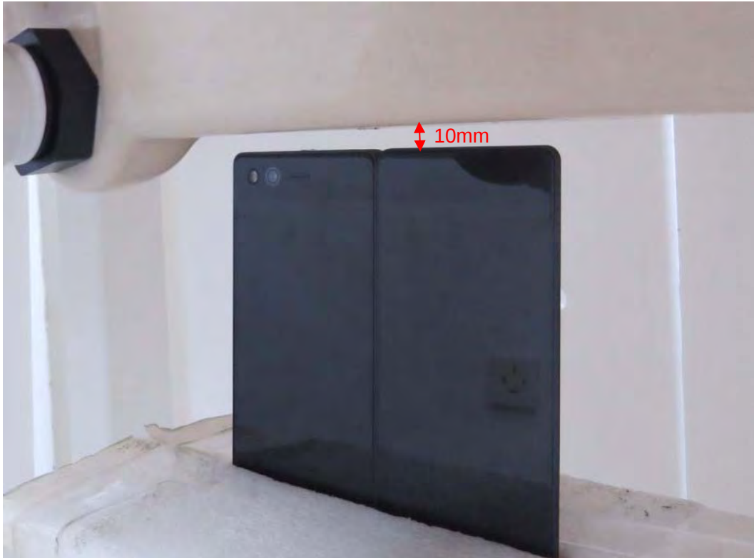
Picture 26: Top Side, the distance from handset to the bottom of the Phantom is 10mm For Double Screen Mode
