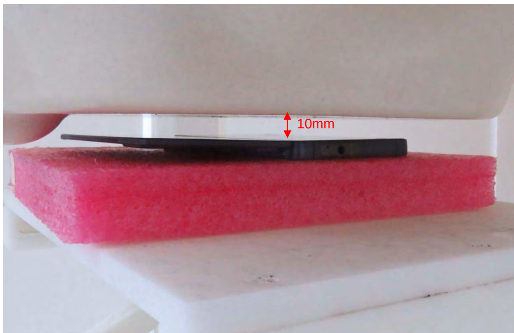
Picture 23: Front Side, the distance from handset to the bottom of the Phantom is 10mm For Double Screen Mode
