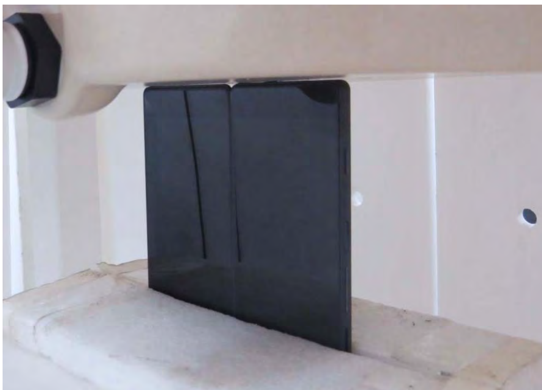
Picture 35: Bottom Side, the distance from handset to the bottom of the Phantom is 0mm For Double Screen Mode
