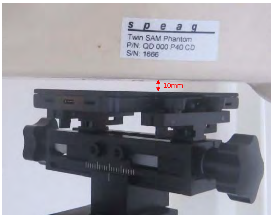
Picture 16: Back Side, the distance from handset to the bottom of the Phantom is 10mm For Single Screen Mode
