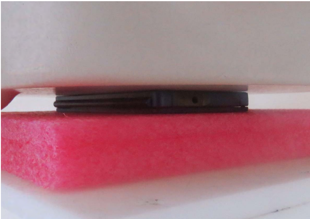
Picture 29: Front Side, the distance from handset to the bottom of the Phantom is 0mm For Single Screen Mode
