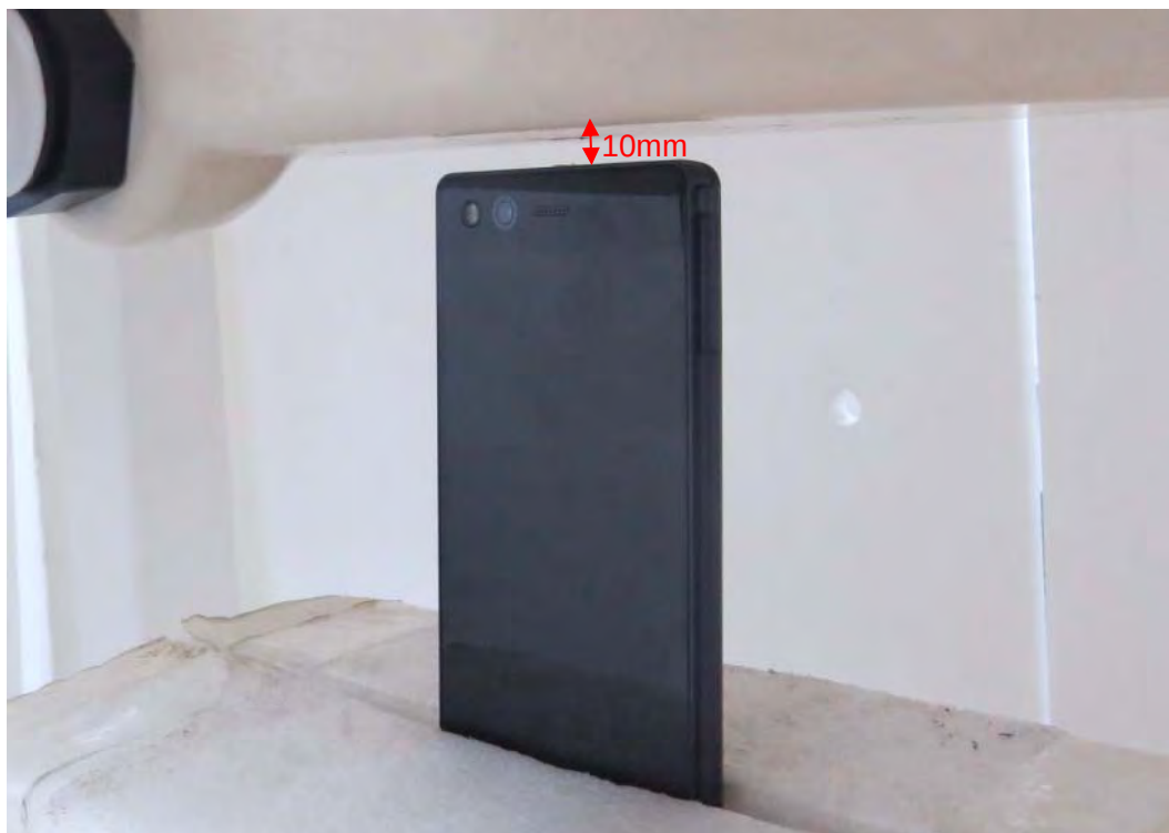
Picture 20: Top Side, the distance from handset to the bottom of the Phantom is 10mm For Single Screen Mode
