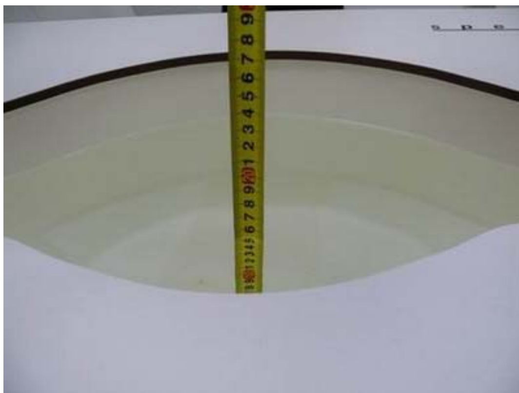
Picture 6: Liquid depth in the flat Phantom (1900 MHz, 15.2cm depth)
