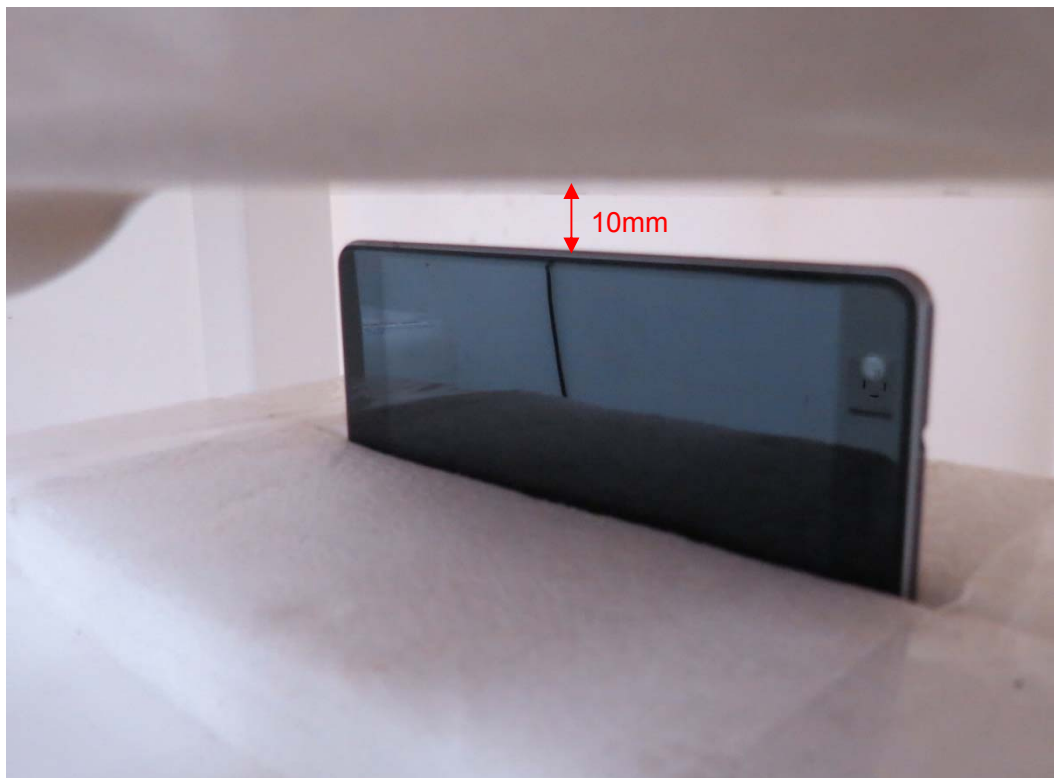
Picture 18: Left Side, the distance from handset to the bottom of the Phantom is 10mm
