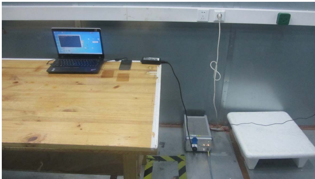
Picture 3 Conducted Emission Test Setup
