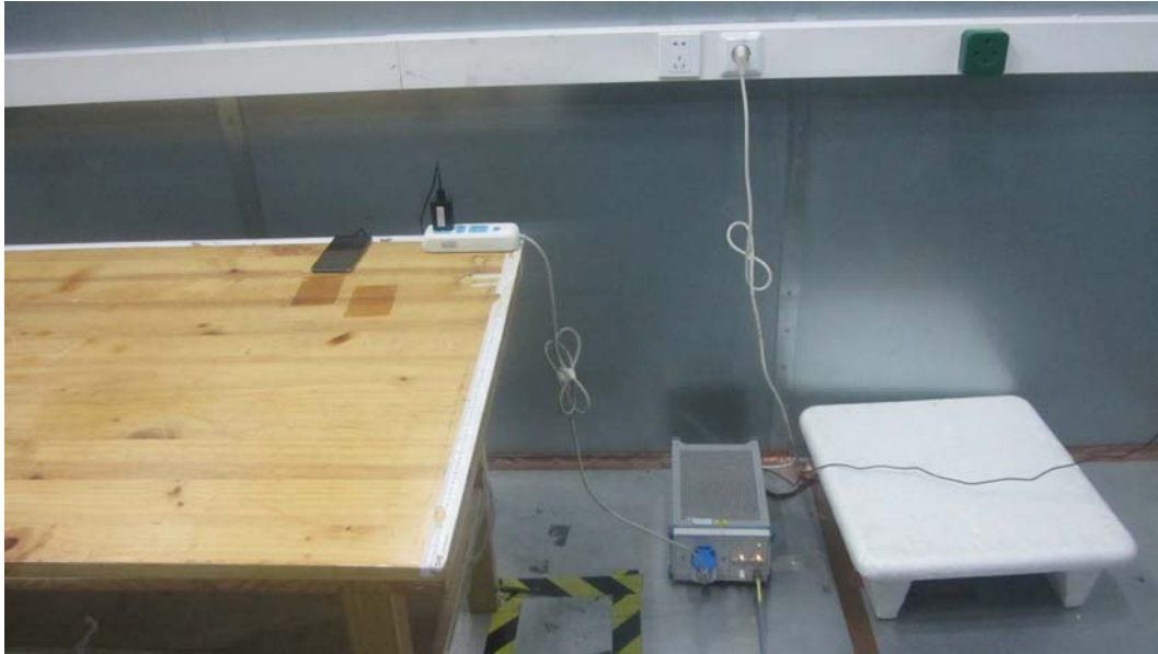
Picture 3 Conducted Emission Test Setup
