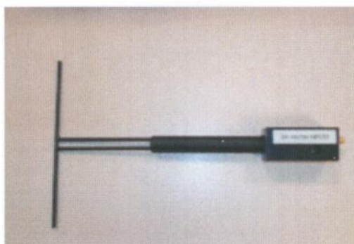
Figure 1 – Satimo COMOSAR Validation Dipole
