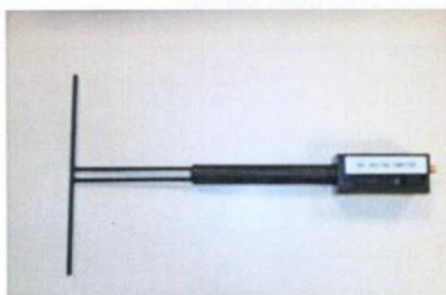
Figure 1 – Satimo COMOSAR Validation Dipole
