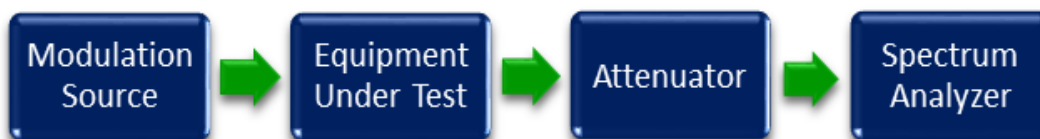
Figure 3: Occupied Bandwidth Test Setup
