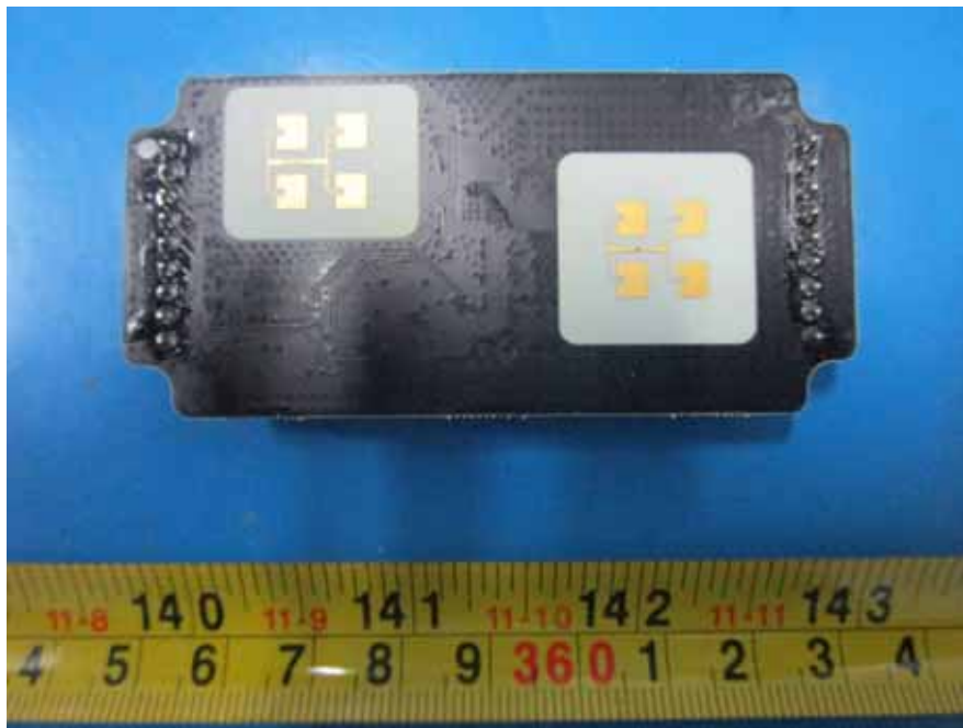
EUT –PCB Top And Antenna View
