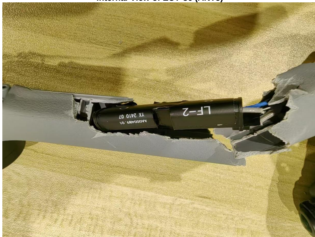
Internal View of EUT-36 (ANT5)
