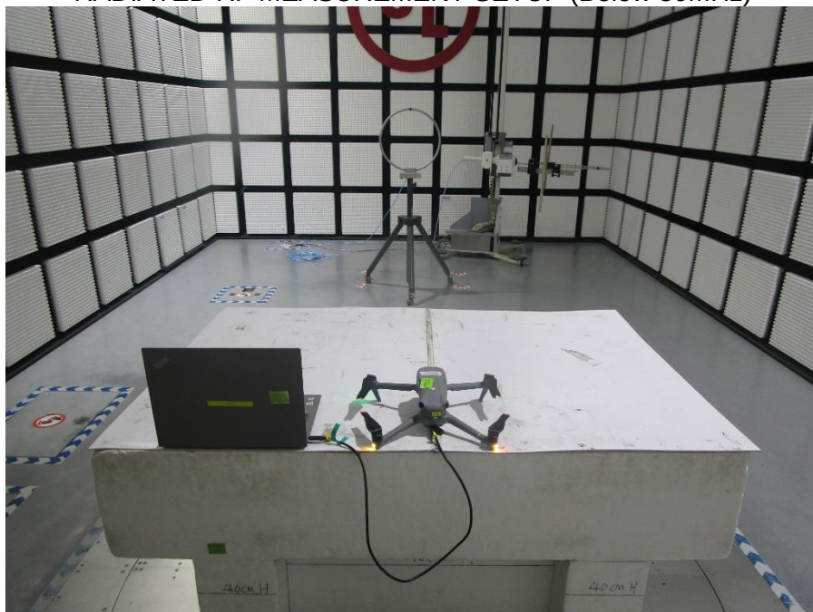
RADIATED RF MEASUREMENT SETUP (Below 30MHz)
