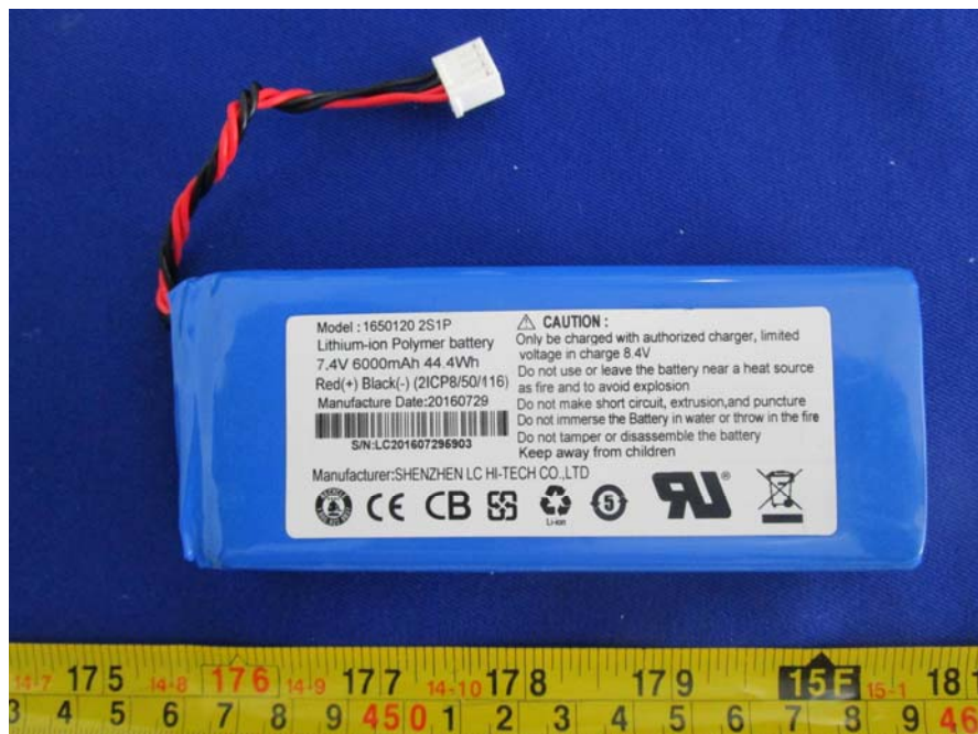
EUT- Battery Top View
