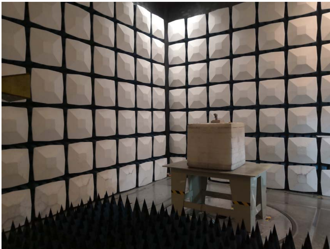
Radiated Emission Above 1GHz View
