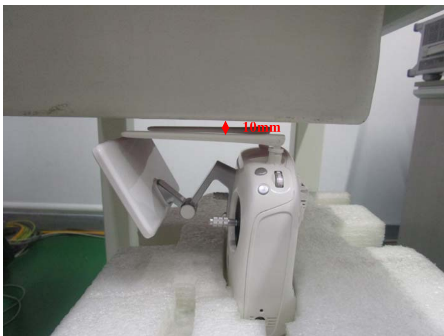
Test Position_Top (10mm)
