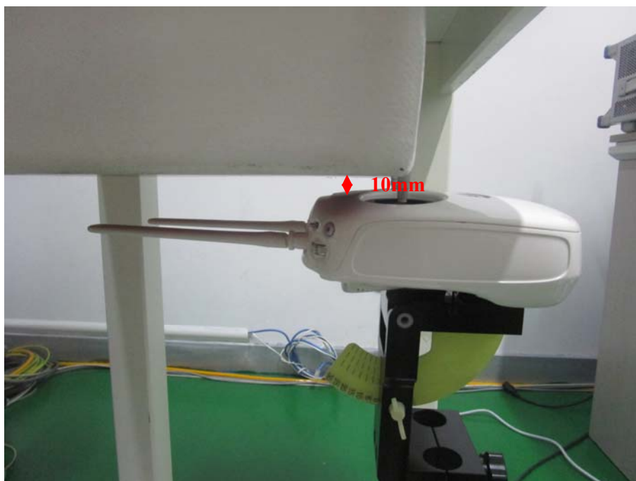
Test Position_Top (10mm)
