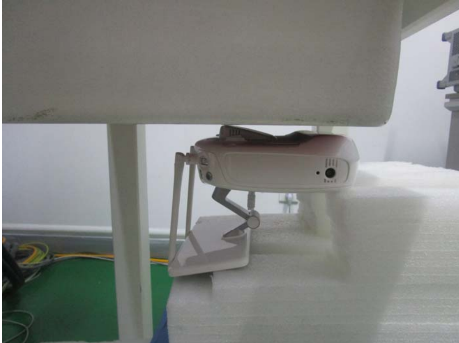
Test Position_Back Antenna Fold (0mm)
