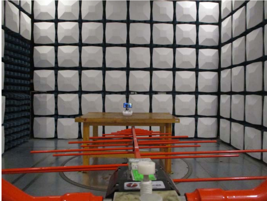
Radiated Emission Above 1GHz View
