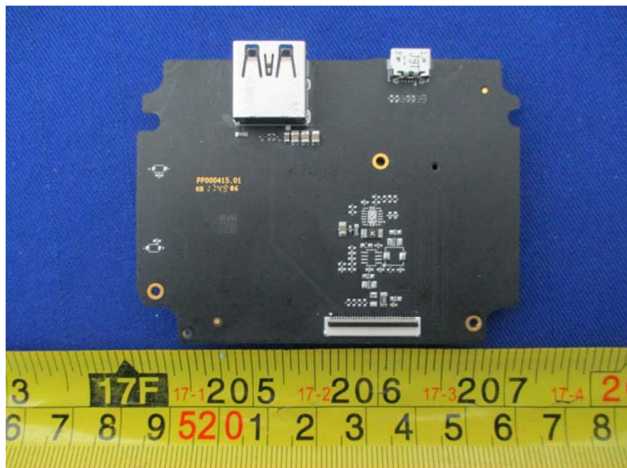
EUT –Power Board Top View
