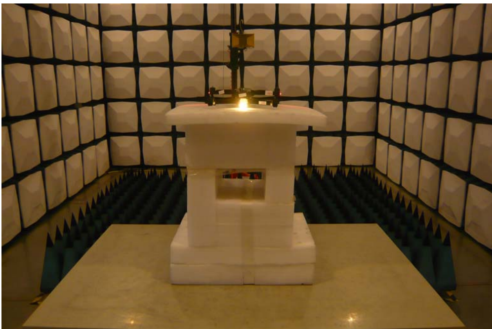
Radiated Emission Above 1GHz View
