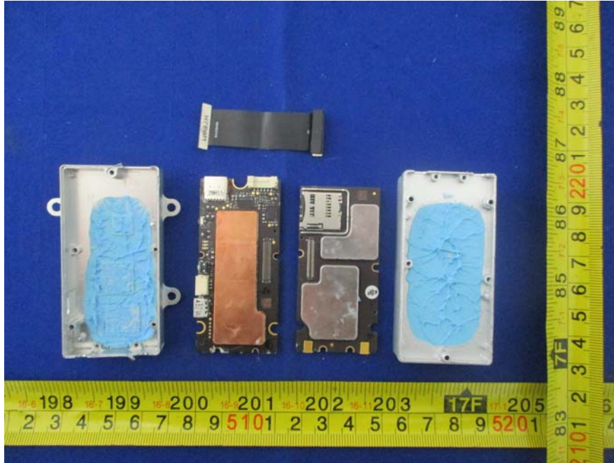
EUT – SDR Module Uncover View
