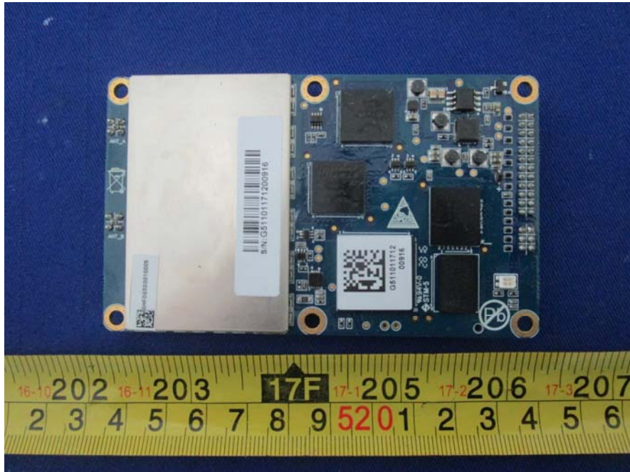
EUT – RTK Module Board Top View
