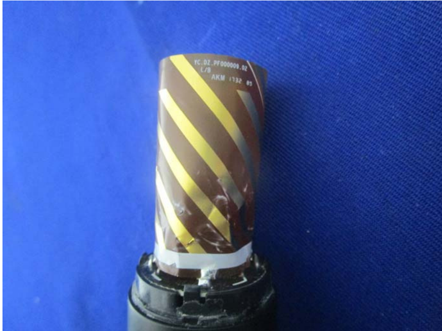
EUT – RTK Antenna View
