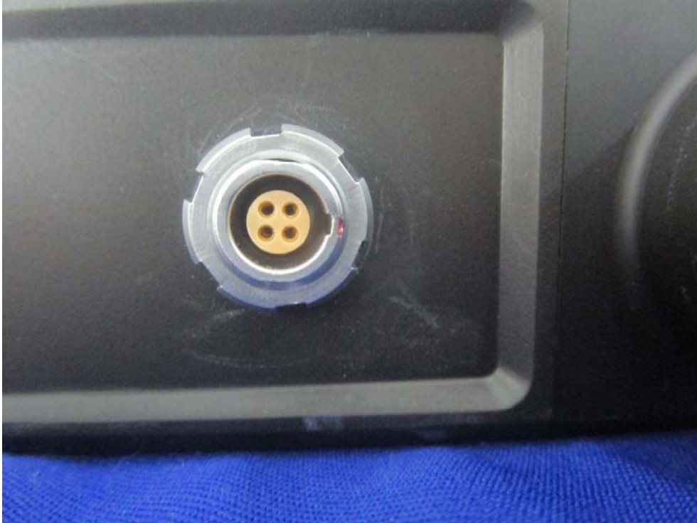
EUT – External Power Port View
