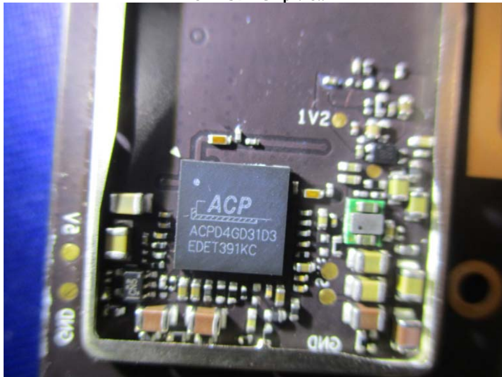
EUT – SDR Chip View
