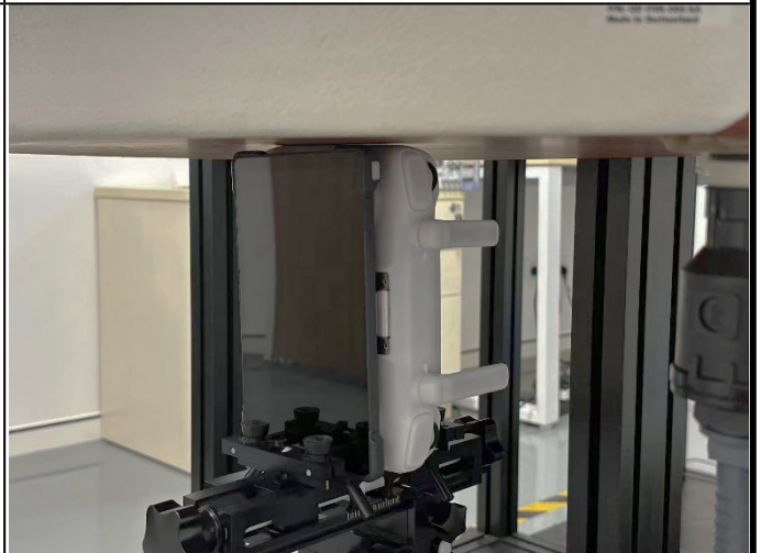
Left Side of EUT with 0cm Gap - SDR ANT0&1_V
