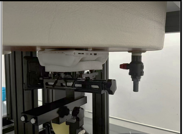
Front Face of EUT with 0cm Gap - SDR ANT0&1_V
