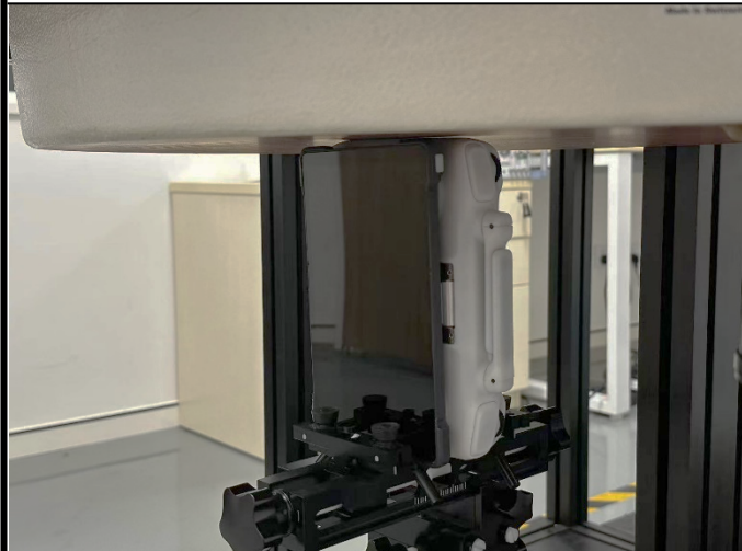
Left Side of EUT with 0cm Gap
