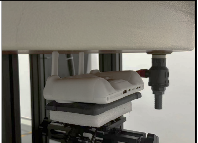
Rear Face of EUT with 0cm Gap - SDR ANT0&1_V
