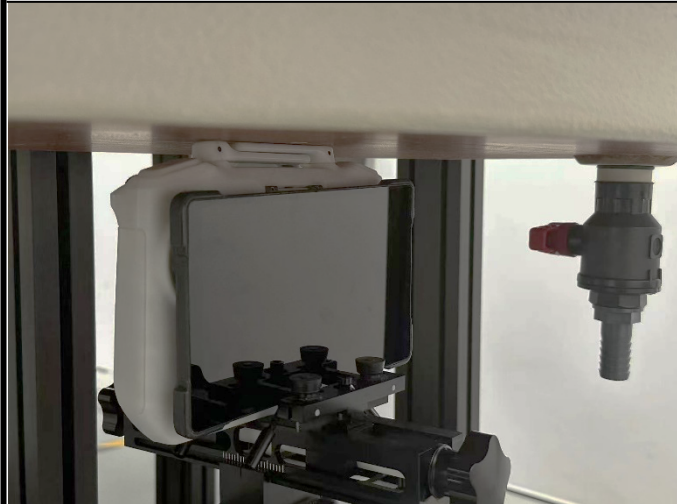
Top Side of EUT with 0cm Gap
