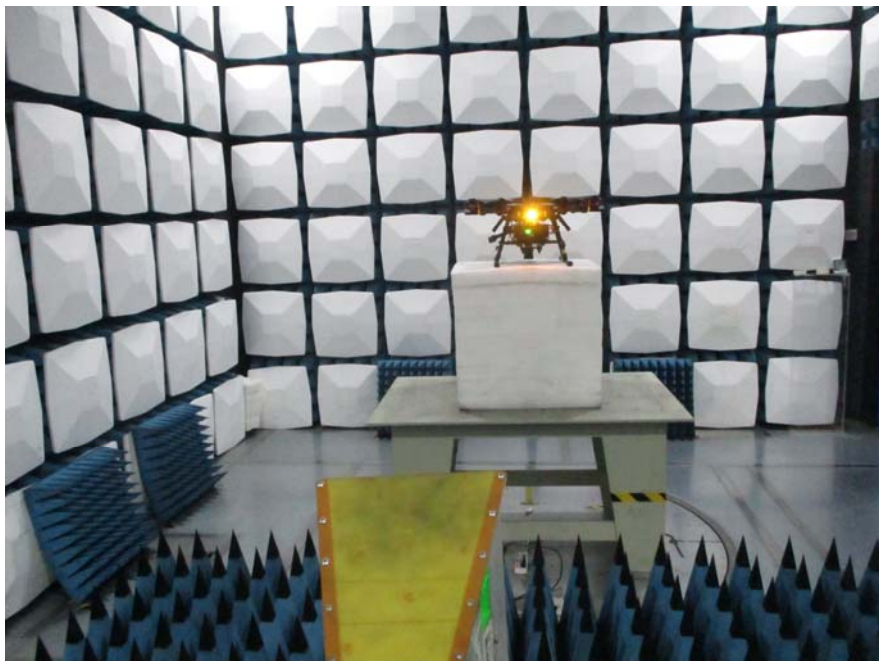
Radiated Emission Above 1GHz View
