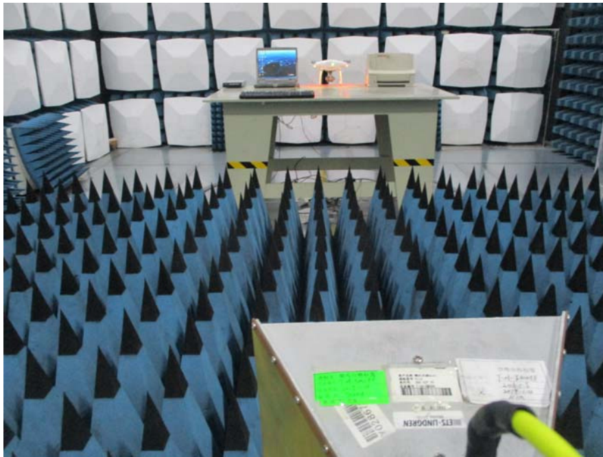
Radiated Emission Downloading Front View (Above 1GHz)
