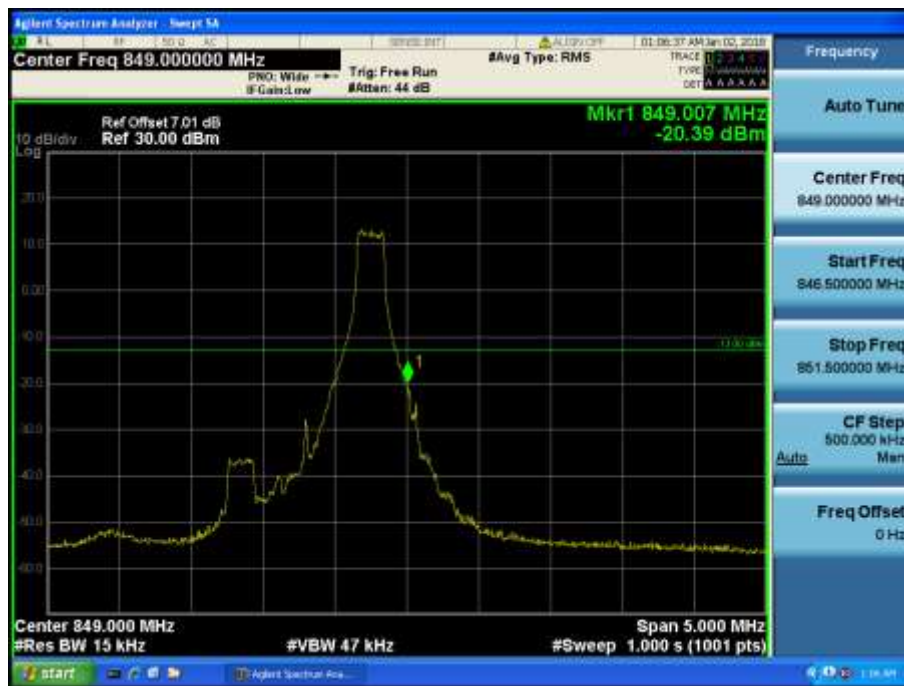
LTE Band 5 / 1.4MHz / 16QAM - RB Size/Offset (1/5)
