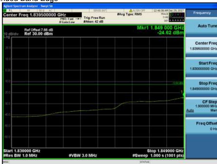
LTE Band 2 / 20MHz / QPSK - RB Size/Offset (50/0)
