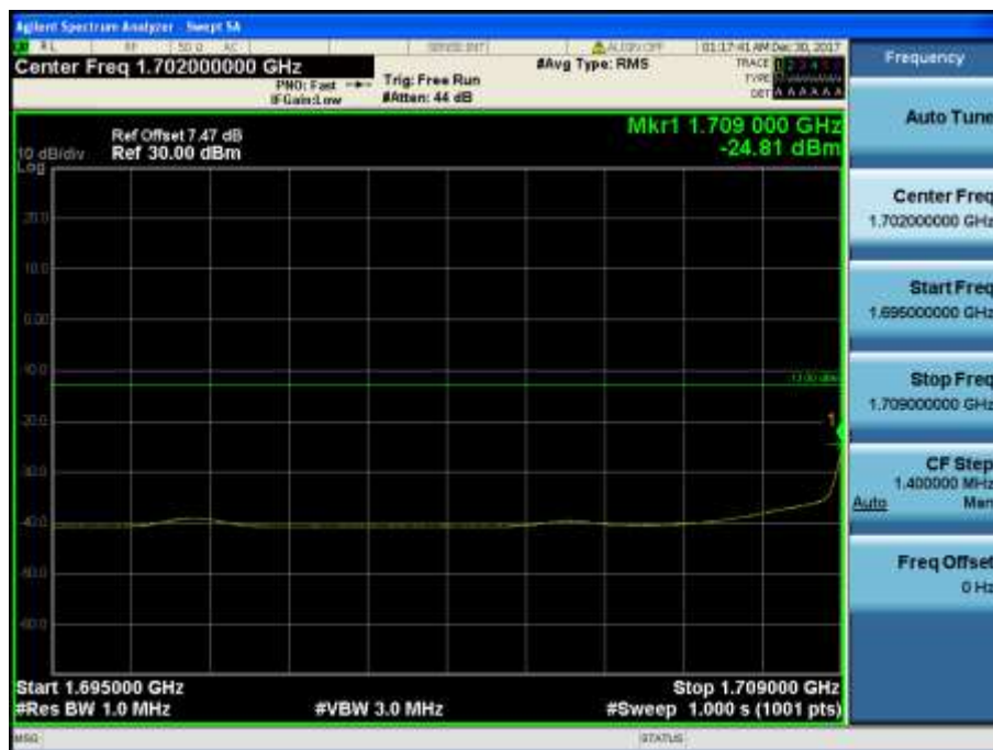
LTE Band 4 / 15MHz / QPSK - RB Size/Offset (1/0)
