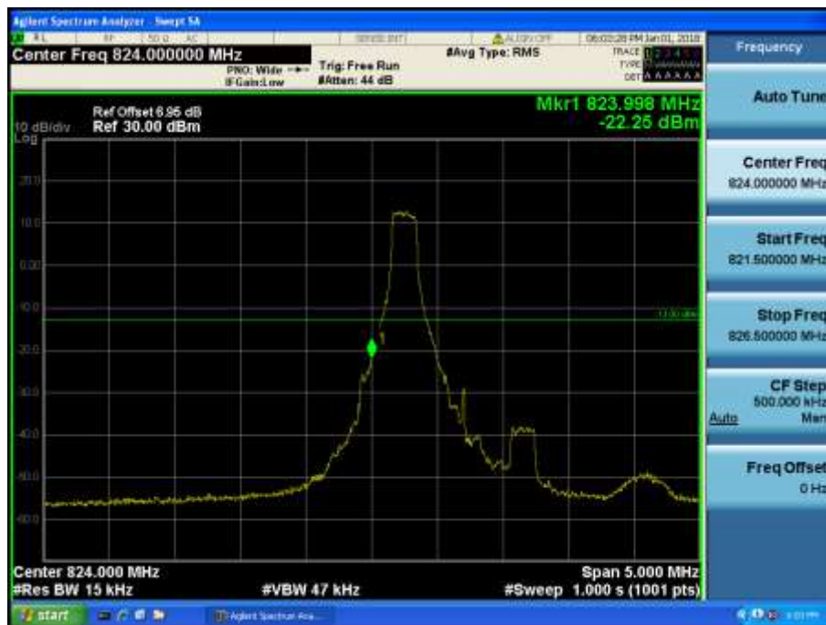
LTE Band 5 / 1.4MHz / QPSK - RB Size/Offset (1/0)
