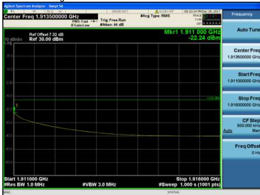
LTE Band 2 / 1.4MHz / QPSK - RB Size/Offset (3/0)
