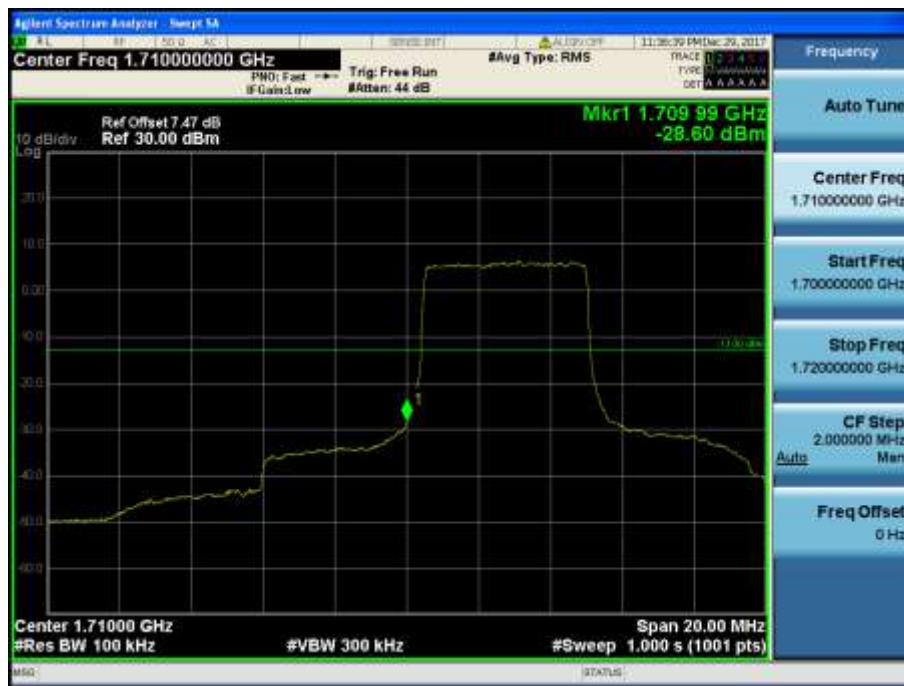
LTE Band 4 / 10MHz / QPSK - RB Size/Offset (25/0)
