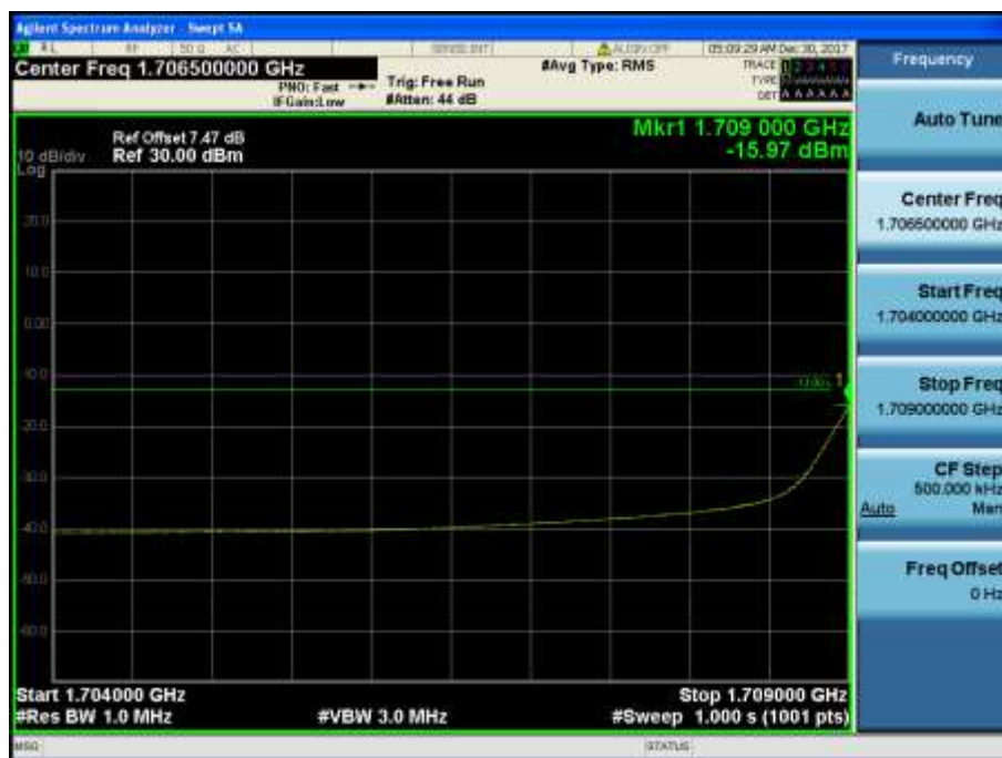
LTE Band 4 / 1.4MHz / 16QAM - RB Size/Offset (3/1)
