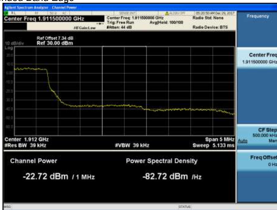
LTE Band 2 / 5MHz / 16QAM - RB Size/Offset (12/13)
