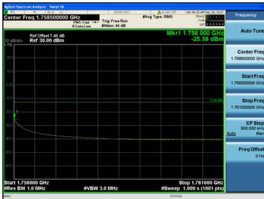
LTE Band 4 / 1.4MHz / 16QAM - RB Size/Offset (3/0)
