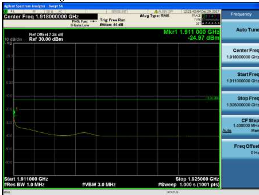
LTE Band 2 /15MHz / QPSK - RB Size/Offset (1/74)
