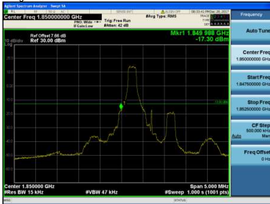
LTE Band 2 / 1.4MHz / QPSK - RB Size/Offset (1/0)
