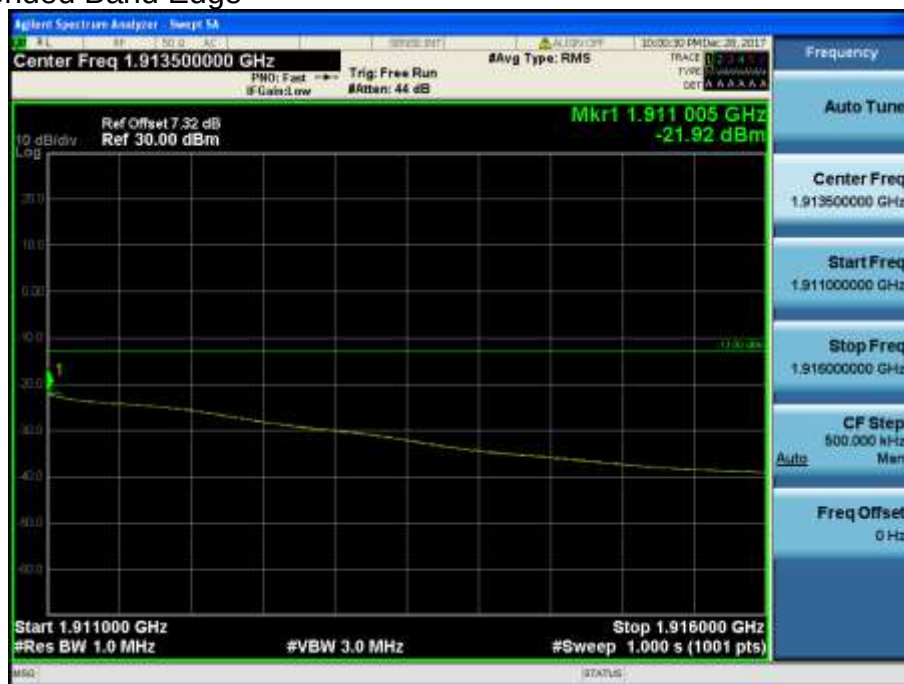
LTE Band 2 / 3MHz / QPSK - RB Size/Offset (8/3)
