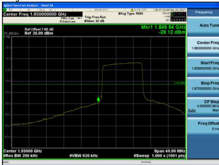
LTE Band 2 / 20MHz / 16QAM - RB Size/Offset (50/0)
