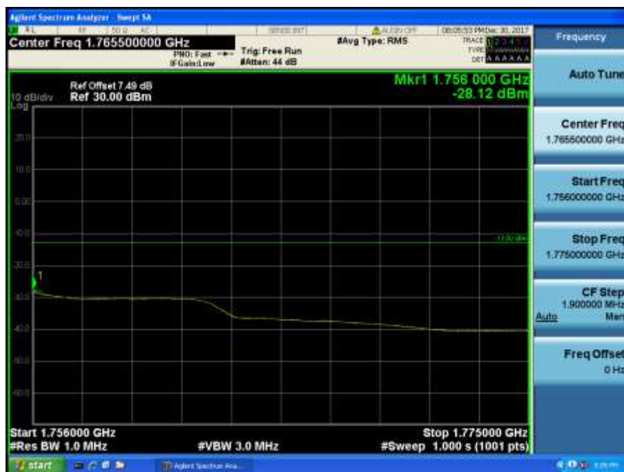
LTE Band 4 / 20MHz / 16QAM - RB Size/Offset (50/50)
