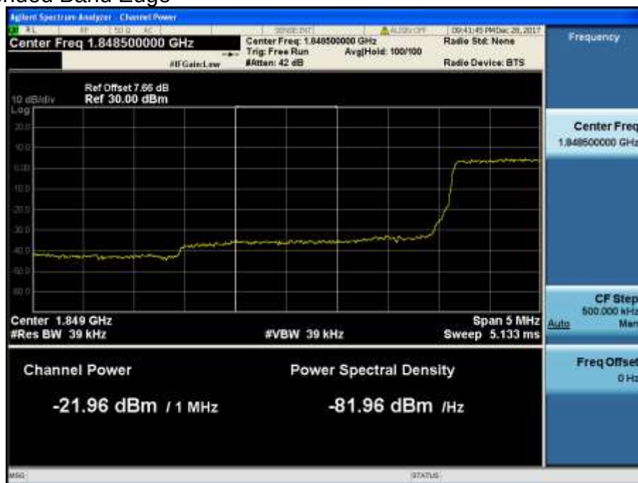
LTE Band 2 / 3MHz / QPSK - RB Size/Offset (15/0)
