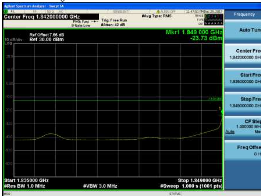
LTE Band 2 / 15MHz / QPSK - RB Size/Offset (1/0)
