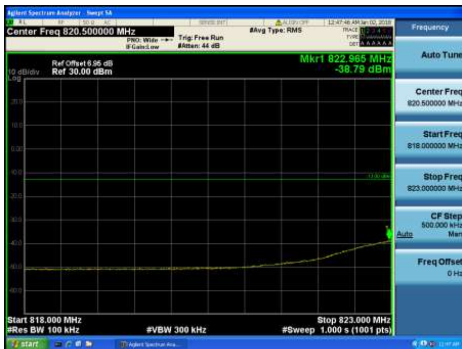
LTE Band 5 / 1.4MHz / 16QAM - RB Size/Offset (6/0)
