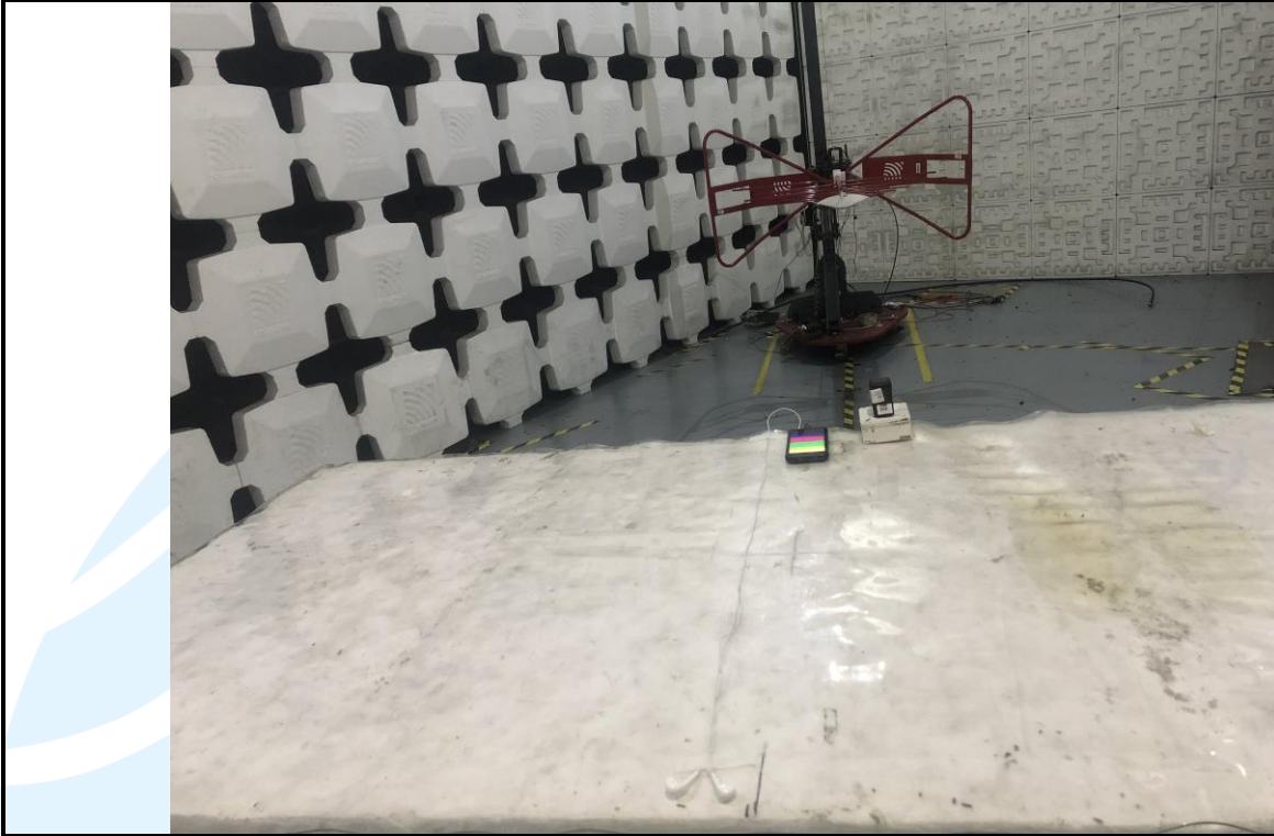
Radiated emission Test Setup-1 (30 MHz~1 GHz)
