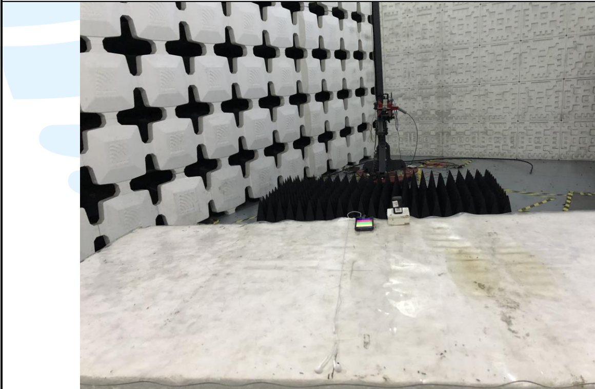
Radiated emission Test Setup-2 (Above 1 GHz)
