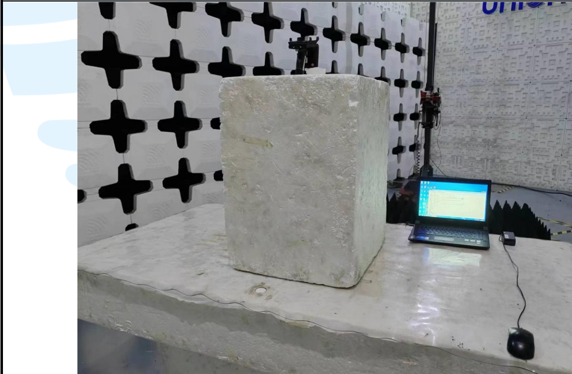
Radiated emission Test Setup (Above 1 GHz)
