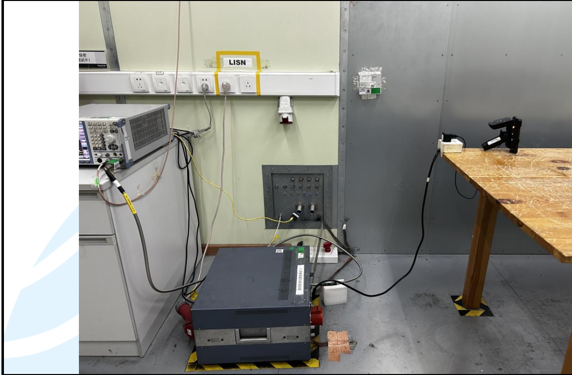
Conducted Emission Test Setup
